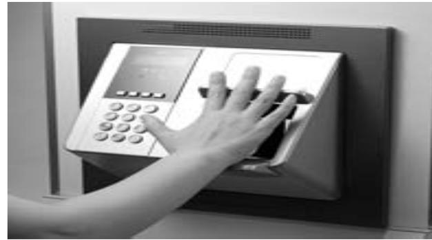
**Figure 3.** ATM with palm vein access control unit pattern authentication sensor unit
