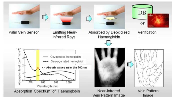
Figure 1 Flow of Palm Vein Technology Process [16].
