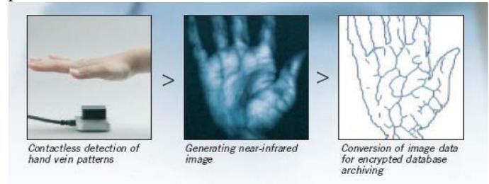
**Figure 2.** Palm Exposure to Sensor and Conversion/ Comparison against from Archival Database
